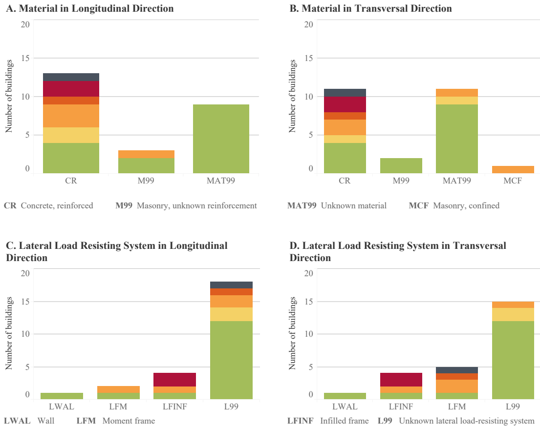
Figure 3.5: Damage grade distribution categorised by adjoining buildings and plan shapes. Material of structural system in (a) longitudinal direction and (b) transversal direction. Lateral Load Resisting system in (c) longitudinal direction and (d) transversal direction.
