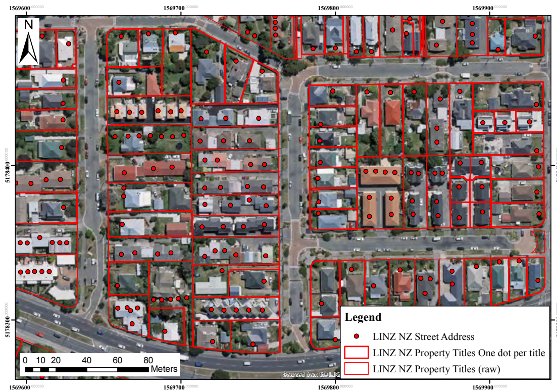
Figure 5.15: Satellite image of urban blocks in Christchurch overlaid with the LINZ NZ Street Address and LINZ NZ Property Titles layers. The polygons with a bold red border represent LINZ NZ property titles having only one street address.
