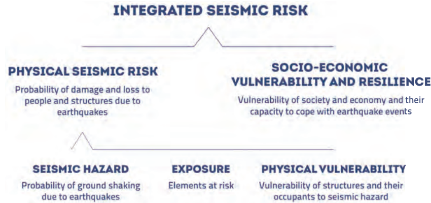
Figure 2. Schematic diagram illustrating the different components of a typical integrated seismic risk model
