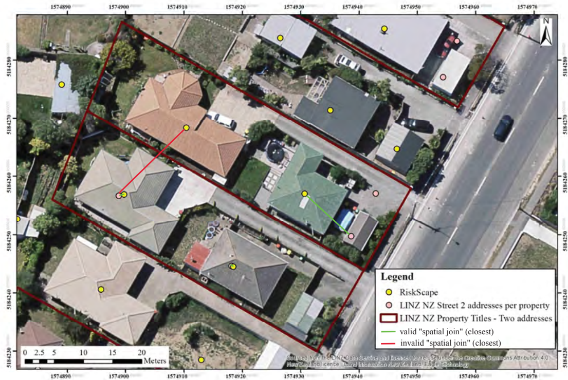
Figure 5.22: Neighbouring properties having two LINZ NZ street addresses and two RiskScope points each leading to issues with the “spatial join - closest”
