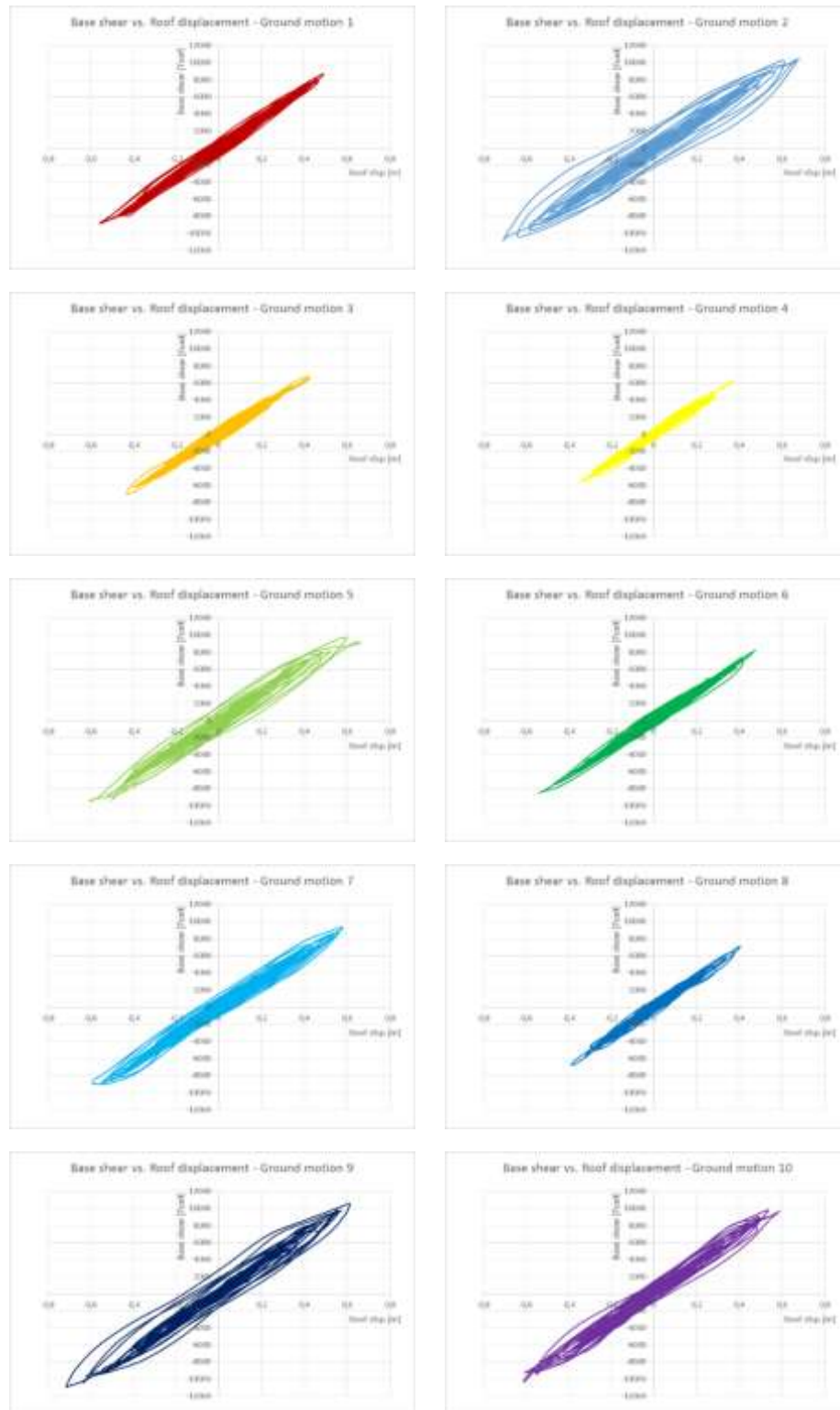
Figure 58: Overview of the base shear vs displacement diagrams for the 10 ground motions
